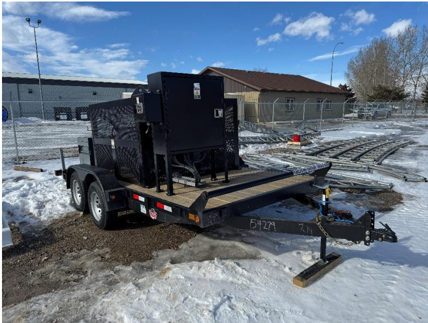
Figure 1: Integral LBX-0001 Mobile Load Box
